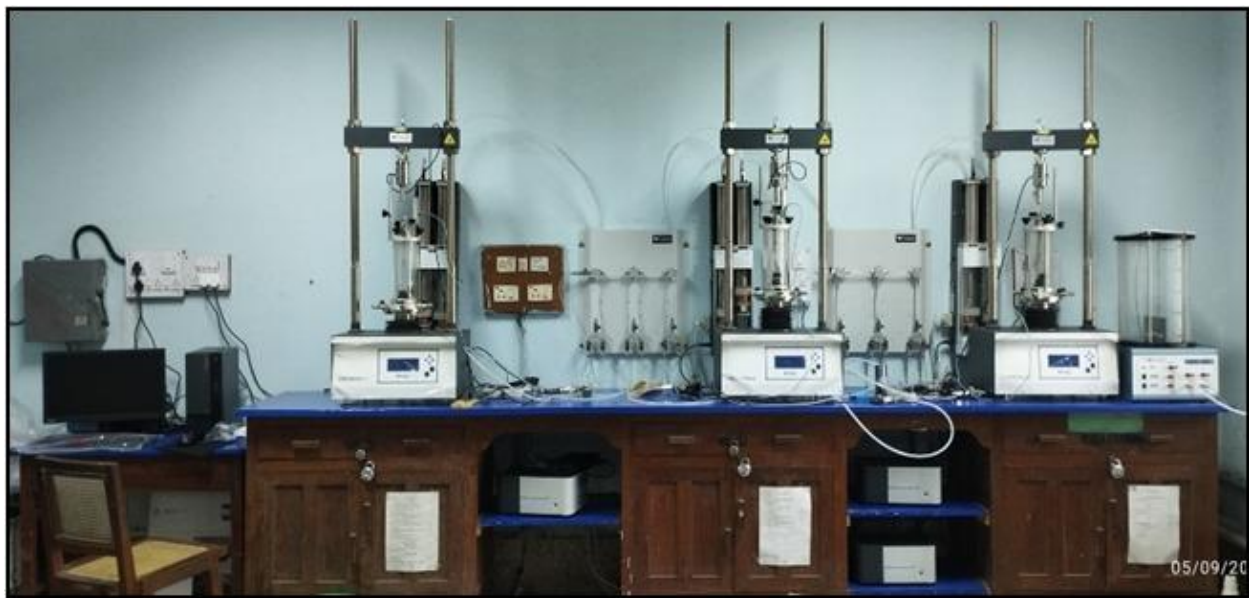
Figure 3.6 Triaxial shear test equipment
