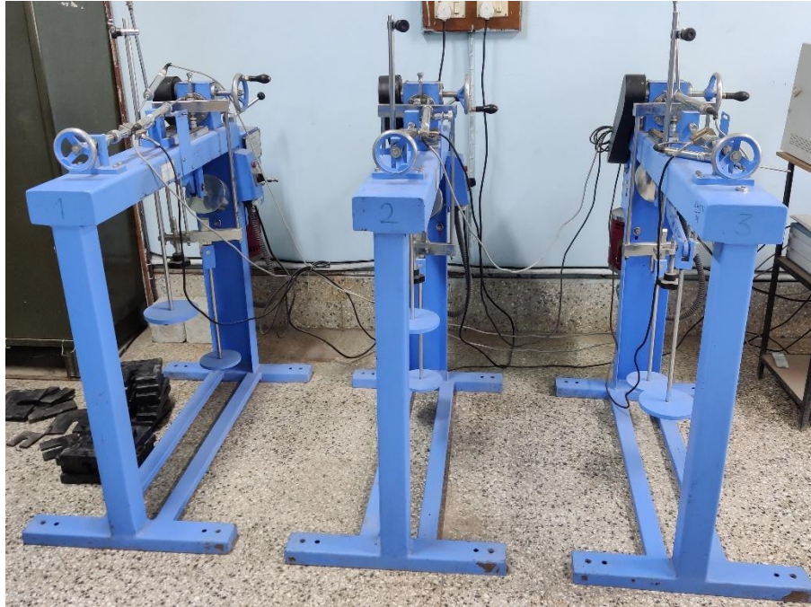
Figure 3.4 Direct shear test equipment
